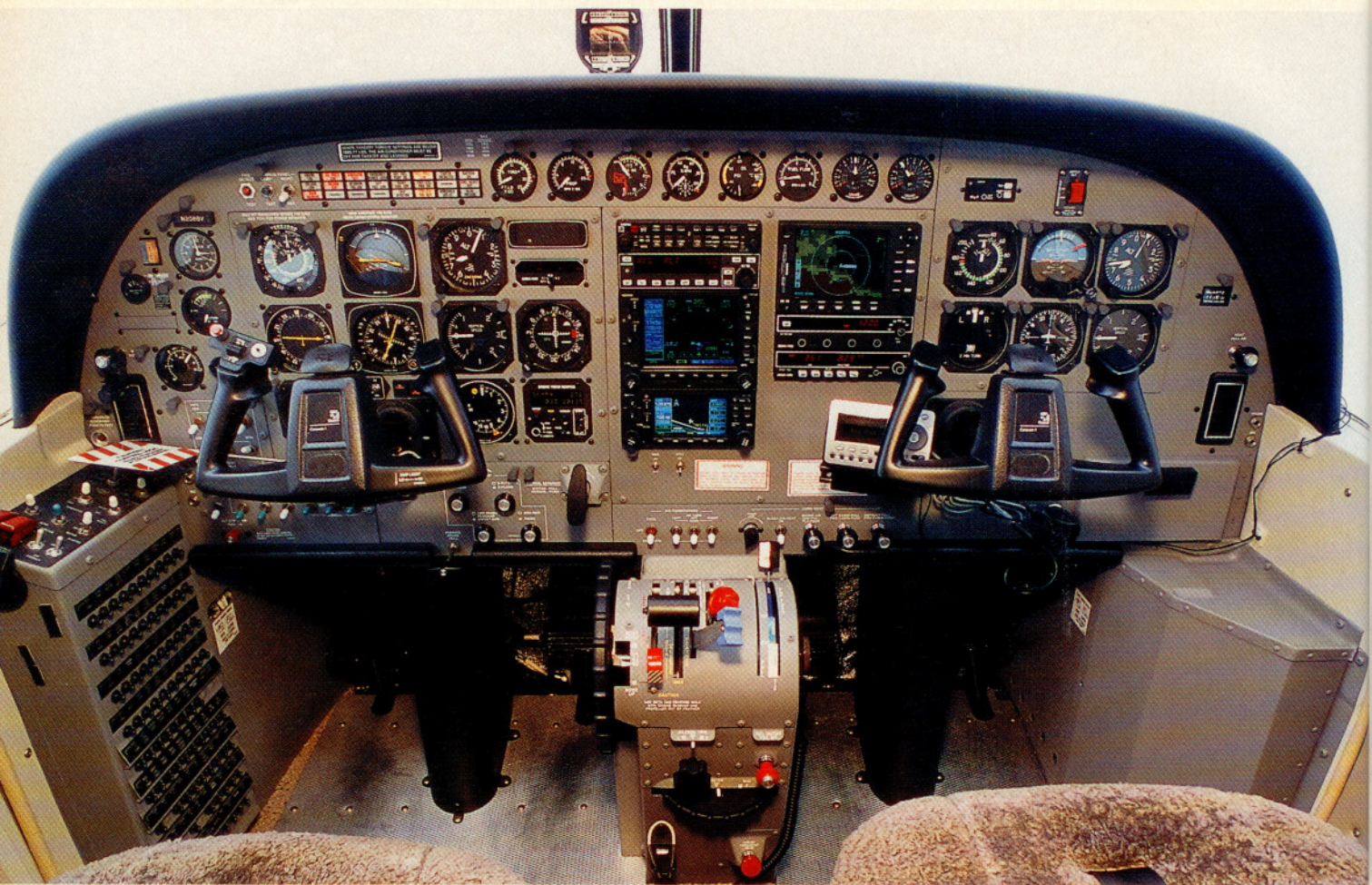
The Bendix/King KMD 880 and Garmin GNS 530 and 430 anchor Vogel's panel (above). Executive seats that articulate to a variety of positions lend an upscale touch to the passenger area (facing page).
